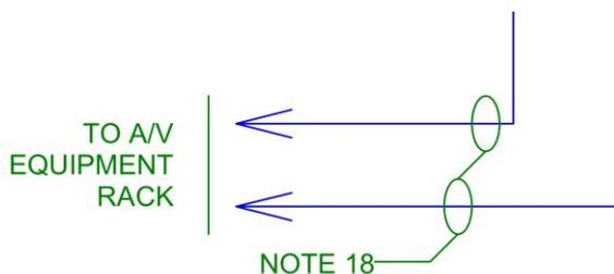
These raceways will typically be terminated at a J-box or wire-trough at the A/V equipment rack location. The A/V J-box and/or A/V wire trough is not indicated on SK-1 (or the DD/CD electrical sheets) as it is typically indicated on the A/V system raceway sheets created by the A/V consultant. The electrical engineer only needs to provide an appropriate note on the E-\* sheets that indicate the raceways are routed to the A/V J-box and/or A/V wire trough. An example of such a note
