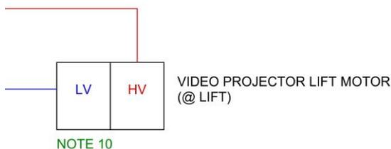
The motor is usually mounted inside the lift case. High voltage connections to the motor are usually brought out to a J-box on the outside of the case, usually on the top. Adjacent to, or part of, this J-box, is a low voltage interface where low voltage control connections can be made.
