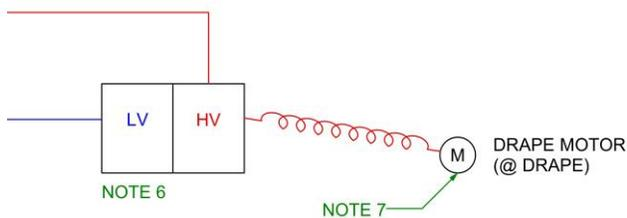
This device is similar to the shade motor controller noted above, but there are many more variables in drapery motor controllers and drapery motors, mainly depending on the size of the drapery and the bulk of the material. Small lightweight drapes/shears may use a small combination motor/controller with high voltage inputs and low voltage control contacts. Medium size drapes may use a small
