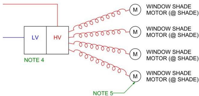
In basic installations, many window shade manufacturers (MechoShade, Vimco, Draper, others) use a Somfy® motor controller, though other similar controllers are available. The device is usually indicated on the electrical sheets as a "GCS" or "MLC" depending on the window shade manufacturer. This device is a NEMA-type enclosure approximately 10" x 10" x 6" deep, has a high voltage section, a low voltage section, and is usually mounted above the accessible ceiling near the window shades.
