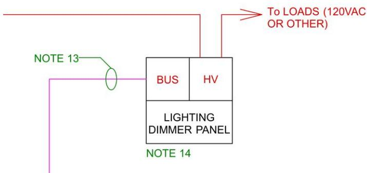
The dimmer panel is usually a large and heavy wall mounted device, the size depending on the quantity of circuits and total dimming capacity. The dimmer panel is usually mounted in a nearby electrical closet or back-of-house utility area.
