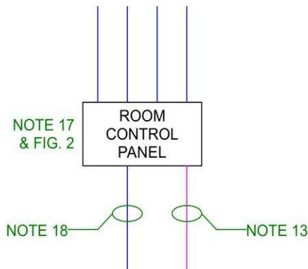
This is a multi-gang box, at least 3" deep, located at project standard switch height on the front or side wall *reasonably* adjacent (with-in 3-4 steps) to the presenters' location. Its function is to locate hard-wired momentary push-button switches to control all of the systems noted above.
