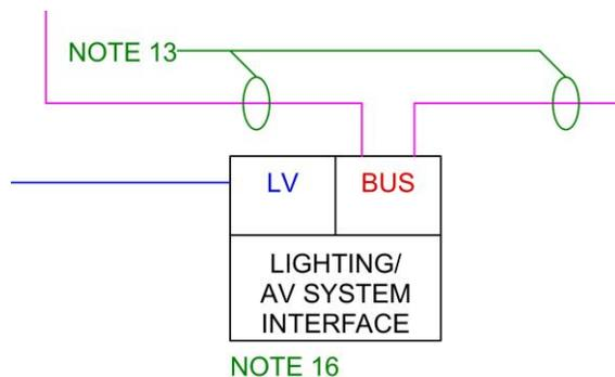
This device allows control of the lighting system by the A/V remote control system. Each dimming system manufacturer employs a proprietary device for this function, but they can be generally characterized as a small J-box with low voltage terminals for the proprietary dimming control bus, and separate low-voltage terminals for connections to the A/V control system.
