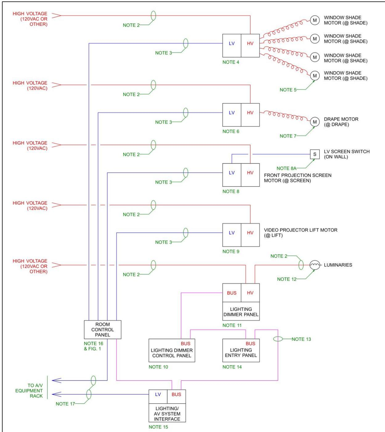
Figure 1: Typical Low-Voltage Systems Cable & Raceway Diagram
