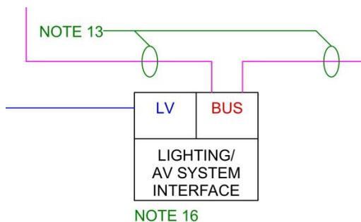
Each dimming system manufacturer employs a proprietary control bus with a unique topology: some use a "star" topology while some use a "series" method; some use shielded twisted pairs, some use individual conductors, some use both. The sequence and topology of devices indicated in the sketch is generic only.
