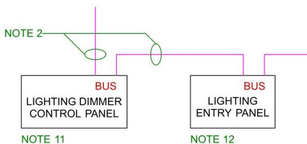
The *dimmer control panel* is a wall-mounted device, usually 3, 4 or 5-gangs that contains the low-voltage control circuitry that adjusts the intensity of each lighting zone. This is accomplished through push buttons (or slide controls) and LED displays to indicate the relative intensity of each zone. There will usually be one control/display for each zone, with a typical panel having up to 8
