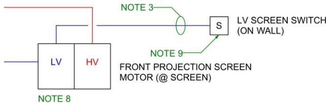
The low voltage control section will typically have screw terminals for contact closures from external switches: one for "Up", one for "Down". Additionally, some manufacturers also provide a third contact for a "Stop" position. As with the window shade or drapery motor controllers, external switches may be push-button, rocker, toggle or any
