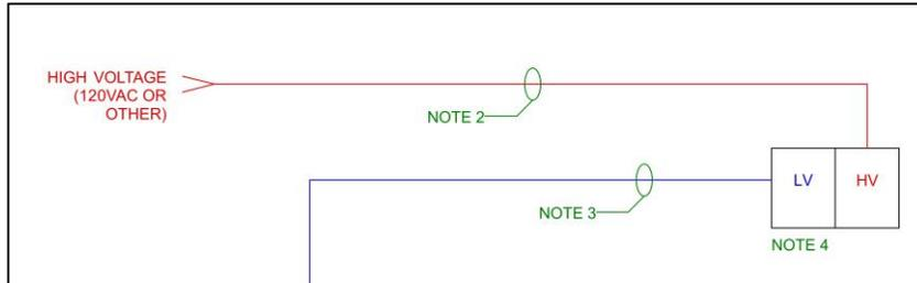
**Note 2:** This raceway and all high voltage conductors provided, installed and terminated under Division 16. This note will be repeated in many of the following diagrams.
